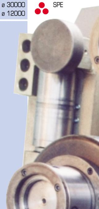
The standard equipment is inclusive of a set of modular rolls, suitable for rolling most of the commonly used commercial sections, such as flats, angles, square and rectangular tubes, Tees, channels, beams.
